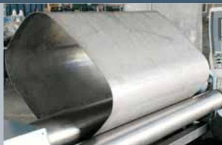
**Conical and poly-centric bendings precisely acquired by control of CNC unit on 4 rolls.**
