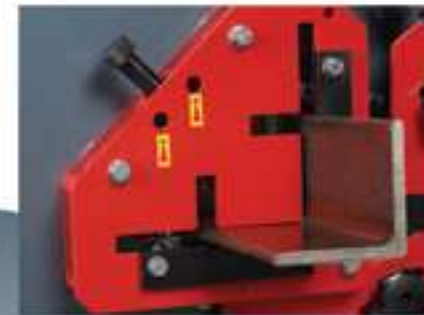
45° miter cut and 90° shearing
