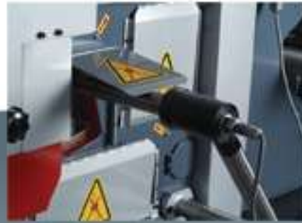
Touch and feel electrical back gauge
