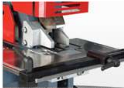
In this station standard rectangular notching and with special blade triangular notching can be performed
