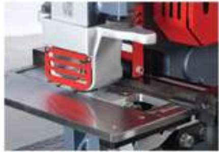
Punching station has max. capacity of Ø27 x13 & Ø18 x18
