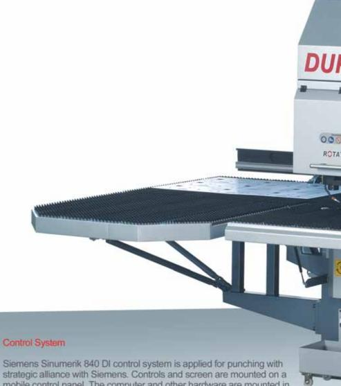
Siemens Sinumerik 840 DI control system is applied for punching with strategic alliance with Siemens. Controls and screen are mounted on a mobile control panel. The computer and other hardware are mounted in a separate cabinet. Machining can be started with just a few steps. Network (Ethernet or RS 232), COM-Port connection is available as well as programming on the control panel. UPS system prevents the control u nit from the voltage fluctuations and cuts.
